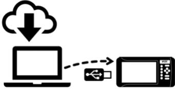
Once all the [tar.gz](#) installer packages have been downloaded, unzipped and copied to the root of a FAT32 USB memory stick, turn the test set's power **OFF**. It must remain connected to the AC/DC charger during the whole upgrade process. Once the upgrade process is started, DO NOT turn it off at any time. The upgrade process will take several minutes, and the test set should reboot itself at the end.
